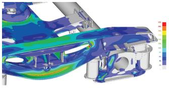
Astra Rail leverages SOLIDWORKS Simulation Premium software to reduce prototyping and testing cycles and optimize designs to reduce weight and increase carrying capacity, and SOLIDWORKS visualization tools to create compelling imagery of new designs.
